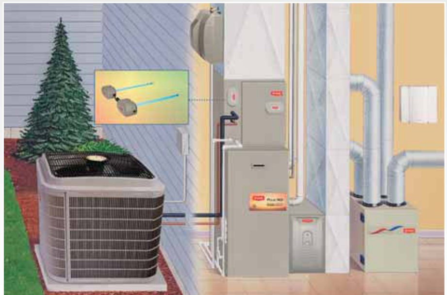
Air Conditioner and Gas Furnace System
